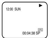
Press COUNTER RESET at the desired tape position. The counter display will be reset to the "00:00:00" position (e.g. the beginning of recording).
